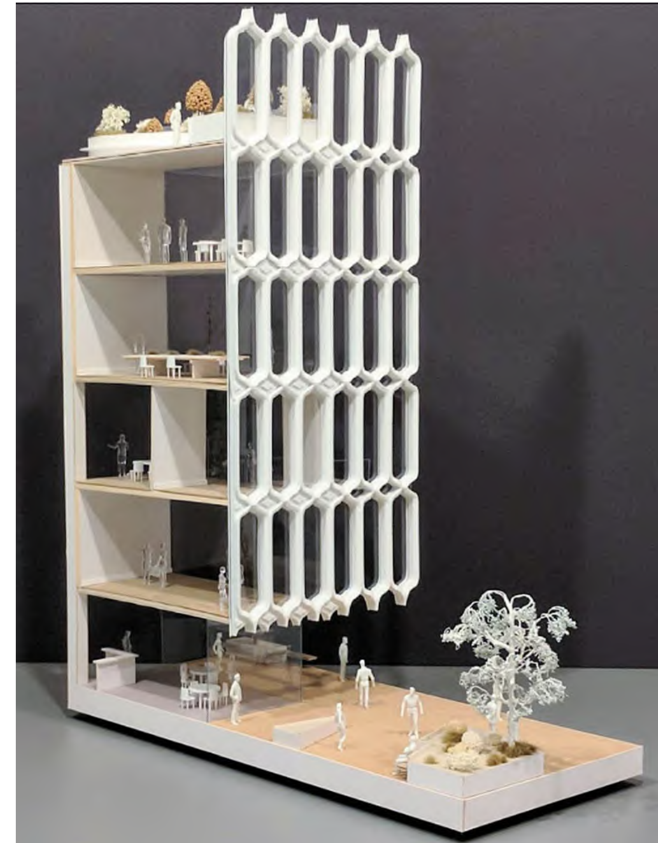
Plot 35 - Sectional model with 3D printed facade 1:50 scale
